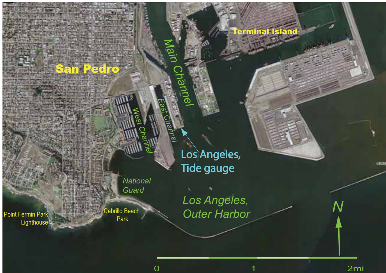
Figure 8: Satellite image of San Pedro Harbor showing the location of the Los Angeles tide gauge used as the reference or warning point for this work. The tide gauge is located on a pier just west of the Port of Los Angeles Main Channel and inside the Los Angeles Outer Harbor breakwater (TerraServer—USA and USGS). The tide gauge is sometimes referred to as the San Pedro tide gauge.
